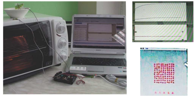
Figure 12: A Bifocal Model for a melting ice cube. The kitchen oven melts the ice (left), and NetLogo both models the phenomena from a differential equations perspective (top right) and agent-based perspective (bottom right).
