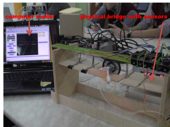
Figure 11: A Bifocal Model for bridge harmonics, with the NetLogo model of a bridge (left), and physical bridge with sensors and a vibrating motor (right).
