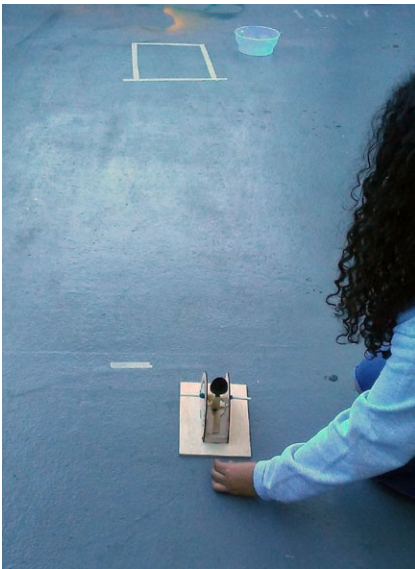
Figure 3 • Student testing her catapult, verifying if the ball lands on the square marked on the floor.
